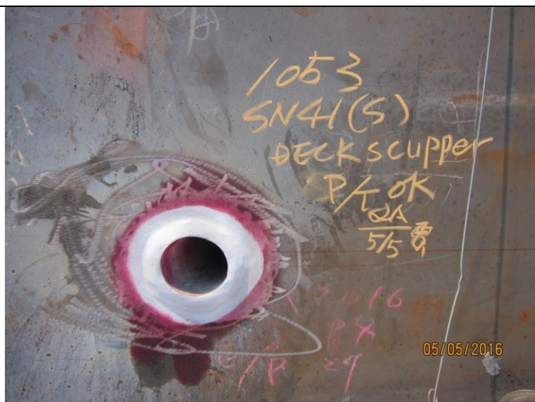
液體滲透劑檢驗法 (Liquid Penetrate Inspection)
