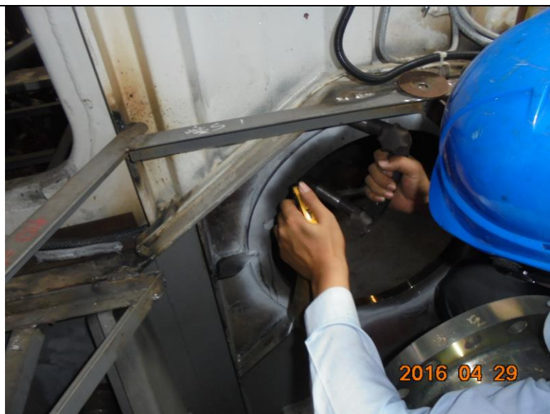
磁粉檢驗法 (Magnetic Particle Inspection)
