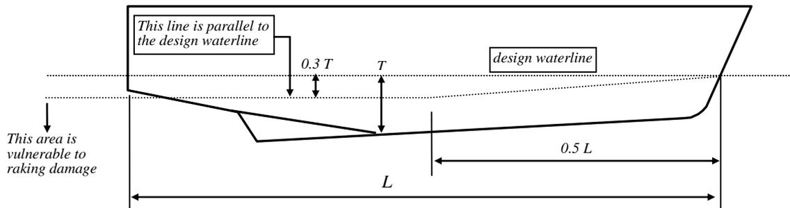
where :  $T$  = maximum draught of the hull (each hull considered individually in the case of multihulls) to the design waterline, excluding any non-buoyant structure, provided that structures such as single plate skegs or solid metal appendages shall be considered to be non-buoyant and thus excluded.
